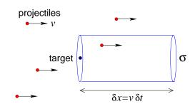
average collision rate per target b  $\Gamma_{per b} = n_a \sigma_{ab} v = \sigma_{ab} j_a$
